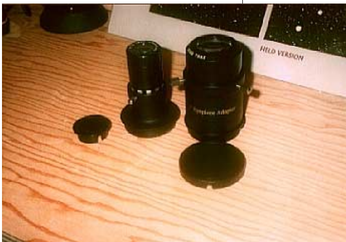
Switching from 2" to 1.25" eyepieces isn't a simple matter of dropping the 1.25"-adapter into the top of the 2-inch adapter. You have to swap one for the other.
