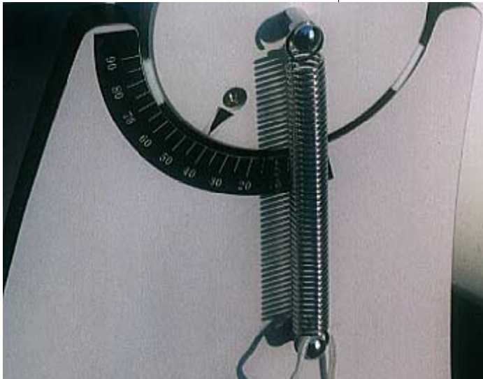
The Spring on each side of the rocker box put enough downward pressure on the Teflon pads to hold the optical tube steady with most eyepieces
