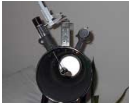
Measuring the focal offset with a Vernier Caliper
