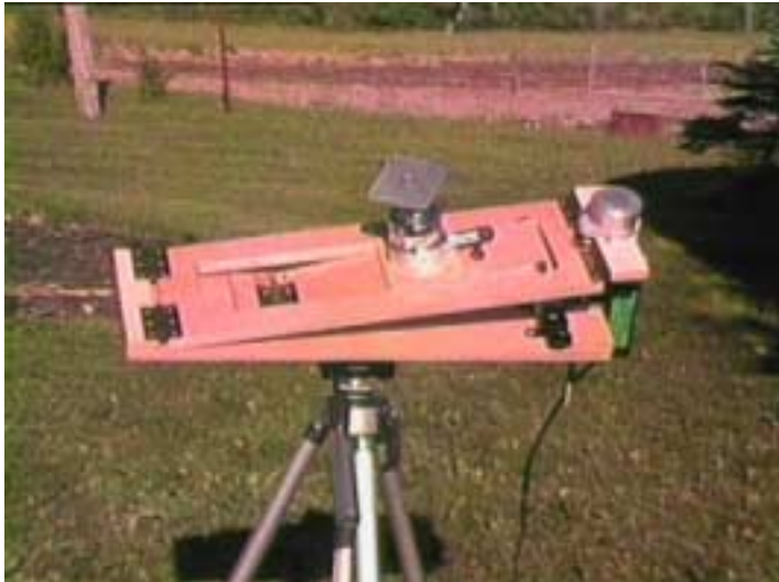
The Completed Barn Door Drive
