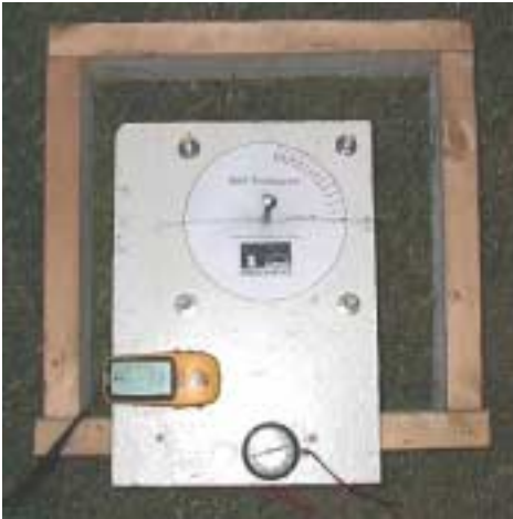
Mounting Template —the sundial face is used to align the mount to true north
